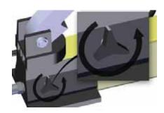
8.2 Remove the Die and Jig from the Pre-Setting head by first unscrewing the Die-Fixing bolt, using the 5mm Hex wrench provided.
