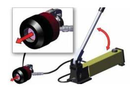
2.5 Open the release valve on the hand pump to retract the Pre-Setting head piston. This action will force any trapped air to move up into the hand pump reservoir.
