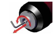
8.3 Remove the Die-Fixing bolt and store in a safe place.
