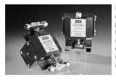
Select HOKE® valves can be remotely actuated. Pneumatic or electric operators provide flexibility and convenience. HOKE® pneumatic actuators feature a unique space saving concept and the ability to operate two valves on the same actuator (pictured). Electric actuators are offered both as weather-proof or explosion-proof units in 115 Volt AC or 24 Volt DC versions.
